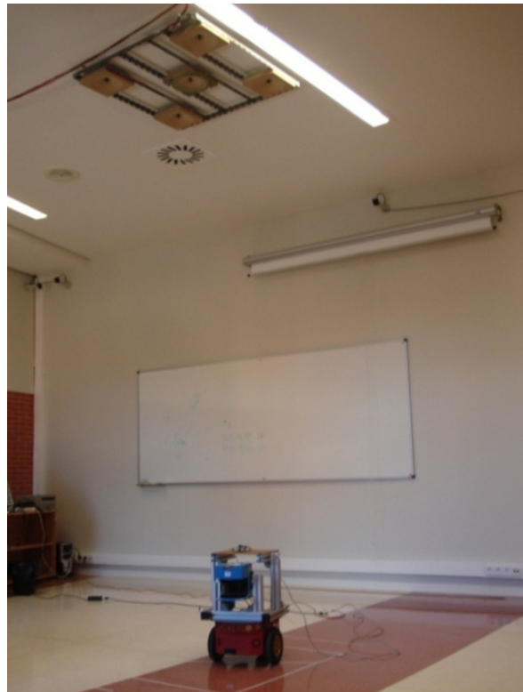
Figure 8. Ultrasonic LPS by GEINTRA used in experimental tests.
