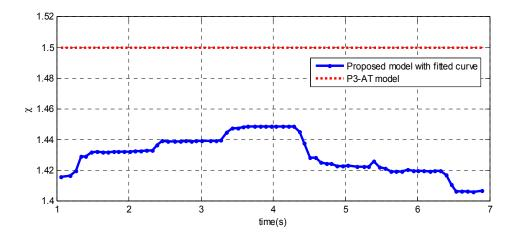
**Figure 16.** ICR coefficient  $\chi$  using the proposed model and the P3-AT model for an example path with the mobile robot.
