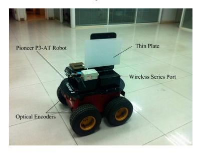
**Figure 6.** Skid-steering mobile robot platform—a Pioneer P3-AT mobile robot.
