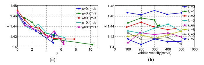
**Figure 12.** The calculated ICR coefficient  $\chi$  for various: (a) path curvatures with  $v = 0.1, 0.2, \dots 0.5 \, m/s$ ; and (b) robot speeds with  $v = 0.1, 0.2, \dots 0.5 \, m/s$  with  $\lambda = 0, 1, 2, \dots, 7$ .
