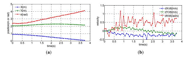
**Figure 11.** Position and velocity of robots calculated by the proposed algorithm. (a) position and heading; (b) velocity.
