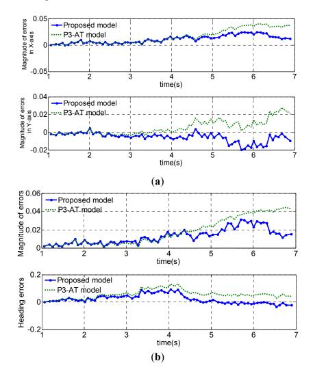
**Figure 15.** Dead-reckoning errors using the proposed model and the P3-AT model for an example path with the mobile robot. (a) Magnitude of position errors in *X* axis and *Y* axis; (b) position magnitude errors and heading errors.
