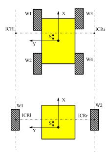
**Figure 2.** Geometric equivalence between the wheeled skid-steering robot and the ideal differential drive robot.
