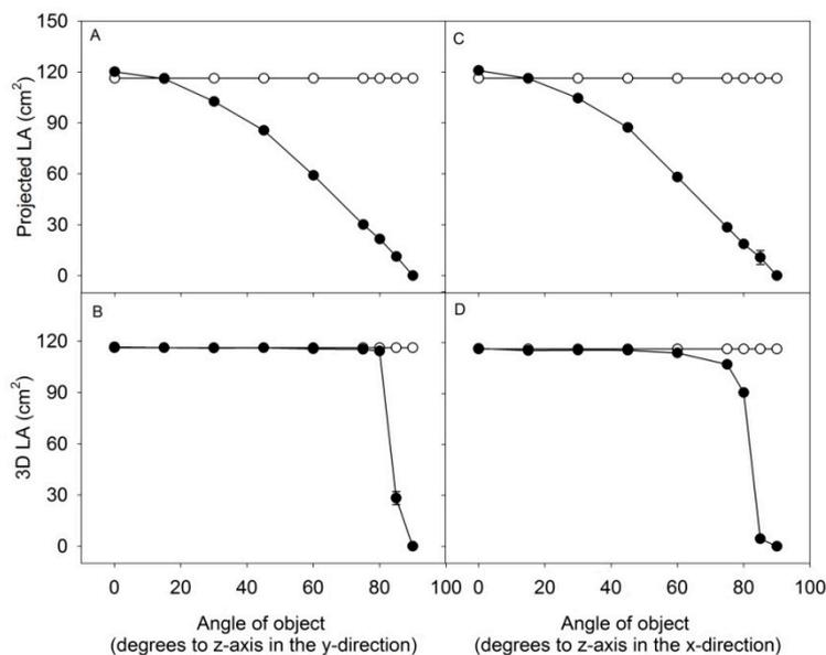
**Figure 3.** An object with defined area of 116.2 cm<sup>2</sup> was tilted stepwise to the z-plane in the y- and x-direction and measured by the 3D scanner. Projected LA and 3D LA of the object was computed at different angles. Area of object (white dots), computed area of object (black dots). Values are average of three  $\pm$  SE, with SE's below 1 cm<sup>2</sup> for most values.
