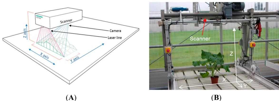
**Figure 1.** (A) Drawing of the 3D scanner, the red lines display the width and projection of the laser line, the blue lines are the projection and width of the camera and the green line/area displays the canopy of a crop stand; (B) The boom system in its starting position with the 3D scanner mounted.
