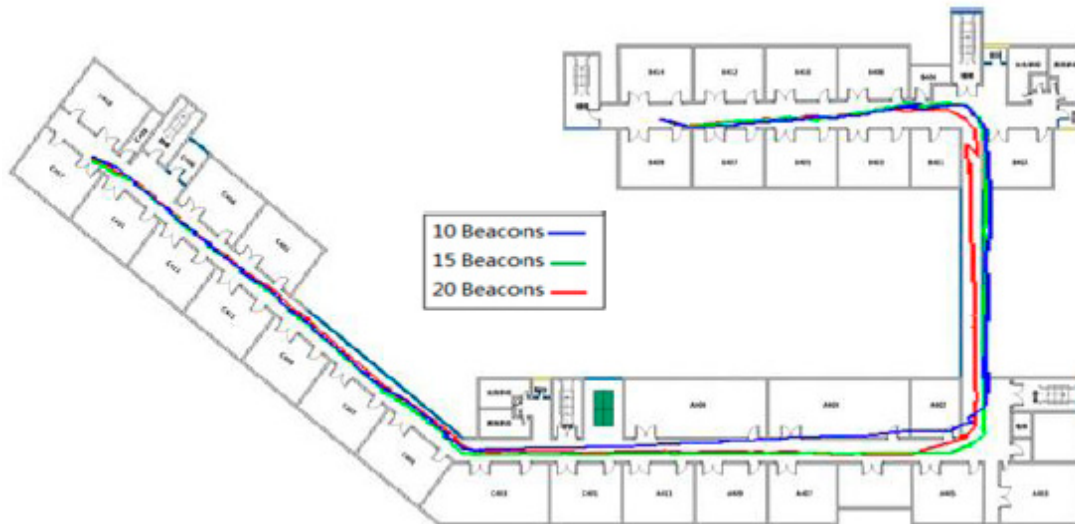
Figure 13. Positioning trajectory analysis for different numbers of Beacons.
