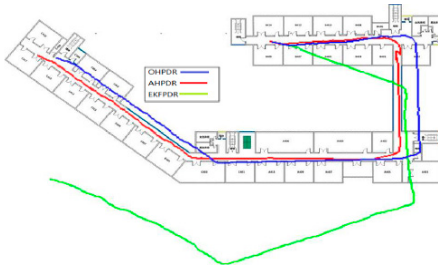
Figure 10. Positioning trajectory analysis for different solutions associated with PDR.
