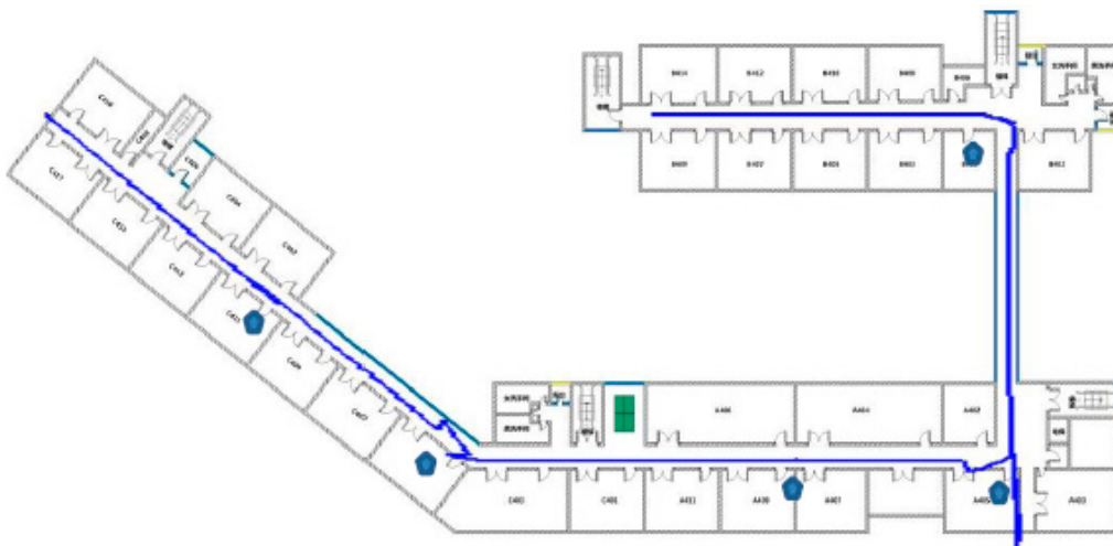
Figure 11. PDR-based positioning method based on map matching with Bluetooth-based position correction.
