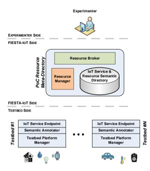
Figure 3. PoC system functional architecture.
