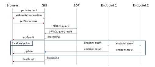
Figure 15. Sequence diagram of the process for retrieving Observations bound to phenomena.
