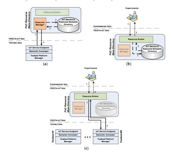
**Figure 4.** PoC system functional use-cases. (**a**) Testbed Resource registration; (**b**) Experimenter Resource look-up; (**c**) Experimenter IoT Service invocation.
