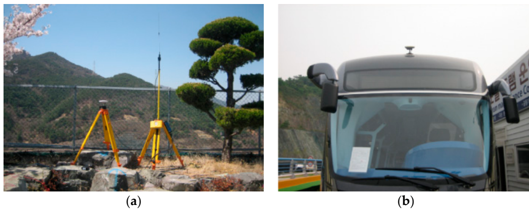
Figure 10. GPS measurement. (a) GPS base station; (b) Rover GPS on the vehicle.
