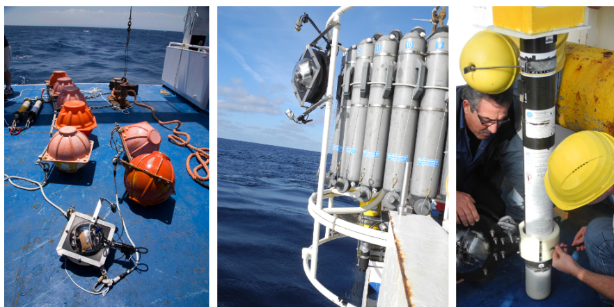
Figure 1. The GUARD1 autonomous imaging system in three of its possible configurations: on the left panel it is hosted on a mooring chain; in the middle panel it is mounted on a rosette; on the right panel it is hosted onboard an ARVOR profiler.
