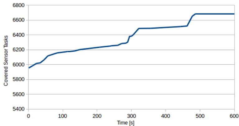
**Figure 7.** How the coverage improves over time. Base (time 0) is greedy solution: coverage 57%. The time limit has been set to 10 min, but the best solution with coverage of 64% was found after 8.1 min.
