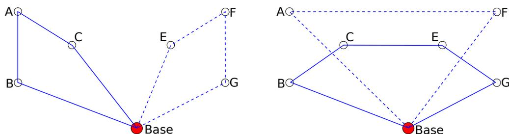
**Figure 1.** Example of planning alternative trajectories of two unmanned aerial vehicles (UAVs) for a task of covering a set of waypoints (A–G). Two possible solutions are shown for both UAVs (solid and dashed lines).
