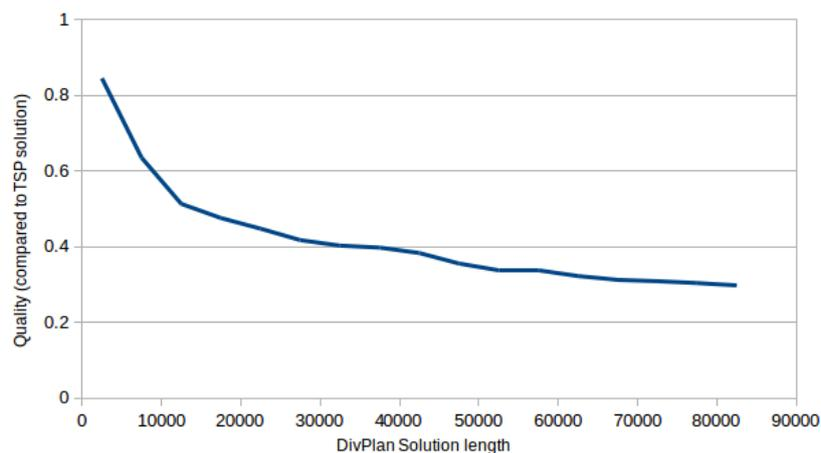
**Figure 3.** Comparison of DivPlan solution with the optimal solution of “omnipotent UAV” covering the same sensor tasks. We can see that the DivPlan solution was in average at most three times longer even for the longest solutions of scenarios with several dozens of UAVs.
