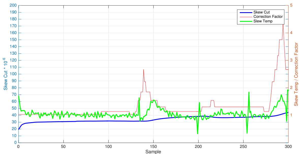
Figure 6. Comparative between skew cut, skew temp and correction factor with temperature variation.
