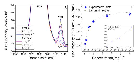
**Figure 3.** (A) Surface-enhanced Raman spectroscopy (SERS) spectra of fluoranthene (FL) detection for concentrations ranging from 0 to 5 mg  $L^{-1}$ ; (B) calibration curve of FL detection (blue circles: experimental data, dotted line: Langmuir adsorption isotherm fit). Insert: zoom on the concentration in the range from 0 to 0.5 mg  $L^{-1}$  (blue circles: experimental data, dotted line: linear fit). The hatched area corresponds to the noise level.
