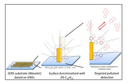
**Scheme 1.** General illustration of nanosensor surface functionalization and preconcentration of the targeted compounds via weak interactions. Gold Nanostructures GNSs, DS-C<sub>10</sub>H<sub>21</sub>, 4-dodecyl benzenediazonium-tetrafluoroborate diazonium salt.
