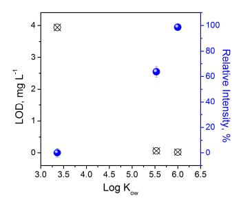
**Figure 6.** Correlation of the limit of detection (LOD) concentration (crossed circles) and the observed related surface-enhance Raman spectroscopy (SERS) intensities of the analytes in the mixed solution (blue circles) plotted as a function of the K<sub>ow</sub> factor of the investigated compounds.
