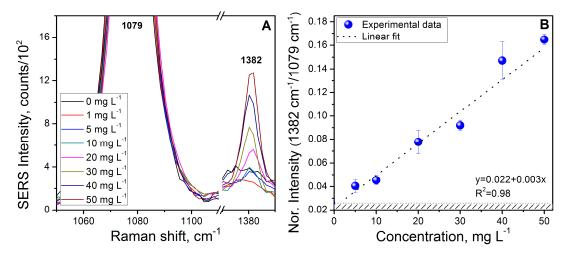
**Figure 4.** (**A**) Surface-enhanced Raman spectroscopy (SERS) spectra of naphthalene (NAP) detection for concentrations ranging from 0 to 50 mg  $L^{-1}$ ; (**B**) calibration curve of NAP detection (blue circles: experimental data, dotted line: linear fit). The hatched area corresponds to the noise level.
