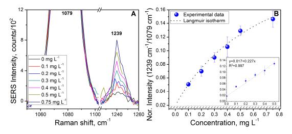
**Figure 2.** (**A**) Surface-enhanced Raman spectroscopy (SERS) spectra of benzo[a]pyrene (BaP) detection for concentrations from 0 up to 0.75 mg  $L^{-1}$ ; (**B**) calibration curve of BaP detection (blue circles: experimental data, dotted line: Langmuir adsorption isotherm fit). Insert: zoom on the concentration range from 0 to 0.5 mg  $L^{-1}$  (blue circles: experimental data, dotted line: linear fit). The hatched area corresponds to the noise level.
