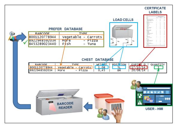
**Figure 8.** Semi-automated procedure related to the insertion of a product with a barcode already known by the HighChest freezer. The "type" information is taken from the "Prefer" database.
