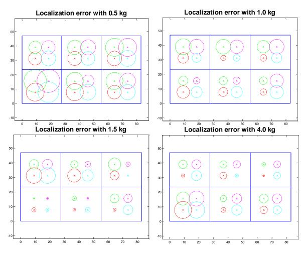
**Figure 10.** Localization error at four points in each of six different compartments for four different object weights. Each error circle was plotted using the Euclidean distance of x and y position errors  $(\sqrt{x_{err}^2 + y_{err}^2})$  as the radius. All errors decreased with increasing weight.
