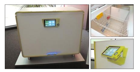
**Figure 1.** The final HighChest smart freezer prototype, showing details of the inner space and user interface.
