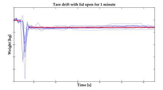
**Figure 11.** Tare drift continuously measured from 5 seconds before opening of the freezer lid to 1 min after lid opening, for 10 repetitions. The pre-opening weight was  $-0.0509 \pm 0.0023$  kg and the post-opening weight was  $-0.6146 \pm 0.0071$  kg. Neglecting the transience due to the effect of manual opening, the average drift due to opening was -0.56 kg.
