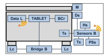
**Figure 3.** Hardware architecture of the sensor- and HMI-augmented chest freezer. The system included an electronic board (Sensors B), connected to internal and external temperature sensors (Ts), a humidity sensor (Hs), a magnet (M) and sensor (Ds) for door status detection, a circuit for monitoring power supply (PSs), a data logger electronic board (Data L), a tablet acting as HMI for the system (TABLET), a barcode reader (BCr), and four load cells (Lc) and their acquisition board (Bridge B).
