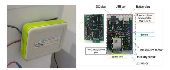
Figure 2. Sensor Board detail from first concept prototype, as well as an architectural description.
