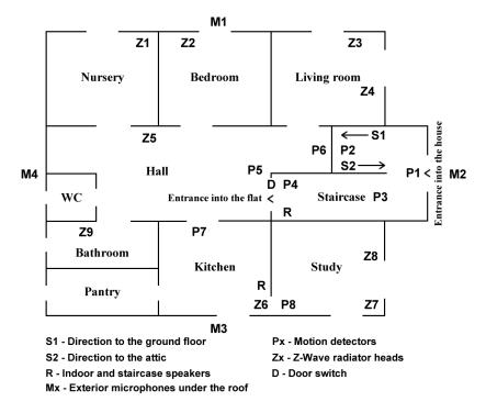
**Figure 2.** Plan of the flat in which a prototype of the system has been installed, and the placement of motion detectors and other input/output components of RUDO system. Source: Authors.
