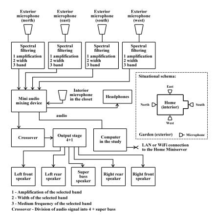
**Figure 3.** Block diagram of the Device Used for Supervising Children Outside (playing in the garden). Source: Authors.
