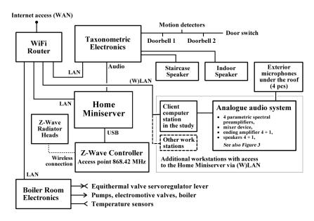
**Figure 1.** Block diagram of the main hardware components of RUDO system. This is the form in which the prototype of the system has been implemented in a detached house. Source: Authors.
