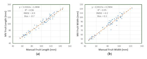
**Figure 5.** Machine vision (MV) and manual caliper measurement of: (a) length; (b) width of mango fruit on tree for the validation set images.
