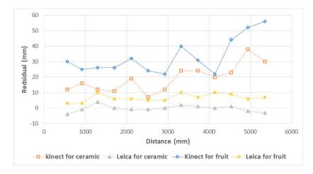
**Figure 4.** Plot of residual of measured to actual distance from device to object as a function of distance to a ceramic tile and to a fruit for Kinect and DISTO technologies (Zed camera results could not be shown on this y scale). Solid lines are used for ceramic measurements, dotted lines for fruit.
