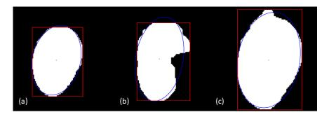
**Figure 2.** Ellipse fitting: (a) An identified well-separated fruit with  $\epsilon = 0.65$  and r = 0.99; (b) failure to fit an ellipse as r = 0.93; (c) failure to fit an ellipse as bounding box (red) length is 4 pixels greater than ellipse (blue) major axis.
