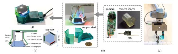
**Figure 12.** The new GelSight fingertip sensor introduced in [29] (©2017 IEEE). The sensor has three LED arrays of different color to illuminate the elastomer surface from a tilted angle of 71°, and a USB web cam to capture real-time image from the sensor. (**a**) the picture of the sensor; (**b**) the schematic diagram; (**c**) the parts of the sensor; (**d**) the sensor mounted on a WSG-50 parallel gripper (Weiss Robotics, Ludwigsburg, Germany).
