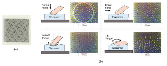
**Figure 3.** (a) an example pattern of printed markers on the GelSight. In the figure, the elastomer is for the fingertip GelSight sensor [30] (Got copyright permission from IEEE), with the dimension of  $25 \text{ mm} \times 25 \text{ mm} \times 2 \text{ mm}$ , the markers have an average interval of 1.1 mm; (b) the markers make diverse motion field patterns under different kinds of forces or torques. The magnitude of the markers' motion is roughly proportional to the force/torque value.
