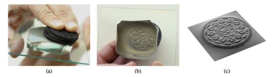
**Figure 1.** (a) a cookie is pressed against the skin of an elastomer block; (b) the skin is distorted, as shown in this view from beneath; (c) the cookie's shape can be measured using photometric stereo and rendered at a novel viewpoint [7] (Got copyright permission from IEEE).
