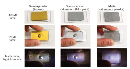
**Figure 4.** Three kinds of elastomer coatings: semi-specular coating painted by bronze flake and aluminum flake paint, and matte coating by aluminum powder. In the second and third row, the three pieces of elastomer are pressed against a ball with diameter of 6 mm, but the in the 3rd row, the elastomer is illuminated by light from side direction.
