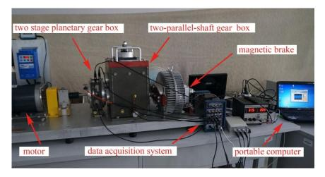
Figure 2. Fault experiment for planetary gear.
