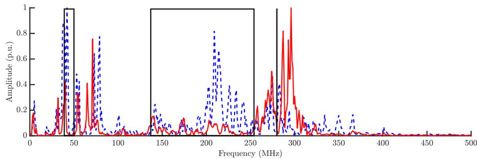
**Figure 8.** Average power spectral density of the signals captured by the antenna 1 and the selected intervals that maximize the distance between clusters in the PR map. The solid line corresponds to dark cluster and the dashed plot to the grey cluster.
