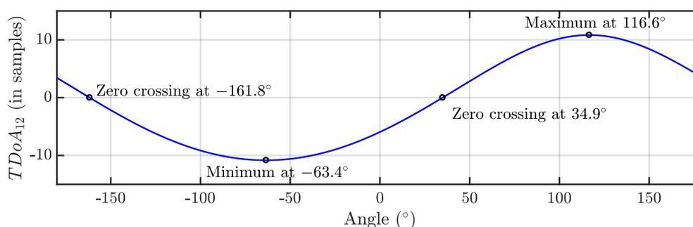
**Figure 3.** Periodic function representing the TDOA vs. the rotating angle. The zero-crossings correspond to the positions of the rig perpendicular to bearing of the source so the distances from the antennas to the source are the same. The maximum and minimum correspond to positions where the rig is parallel to this bearing so one of the antennas is at the farthest relative position with respect to the source and the other at the closest one.
