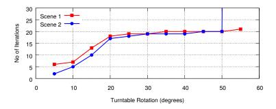
Figure 9. Number of iterations required by the ICP-BD algorithm in two scenes shown in Figure 5 of [24].
