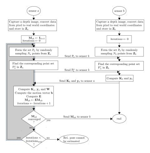
**Figure 4.** Operation of the cooperative relative pose estimation algorithm. The algorithm is distributed over two sensors, and operates iteratively (denoted in gray) until it converges or maximum number of iterations is reached. We have used the convergence criterion presented in [55], and iterations $_{max}$  is set as 50 (see Section 4.1).
