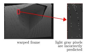
**Figure 8.** Ghost artifacts: the light gray pixels actually belong to the background surface and falsely warped onto the surface at the foreground.
