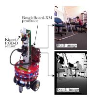
**Figure 11.** eyeBug [69,70], the mobile RGB-D sensor we used in our experiments. The color and depth data generated by the Kinect sensor is processed on a BeagleBoard-xM [71] computer running the GNU/Linux operating system.
