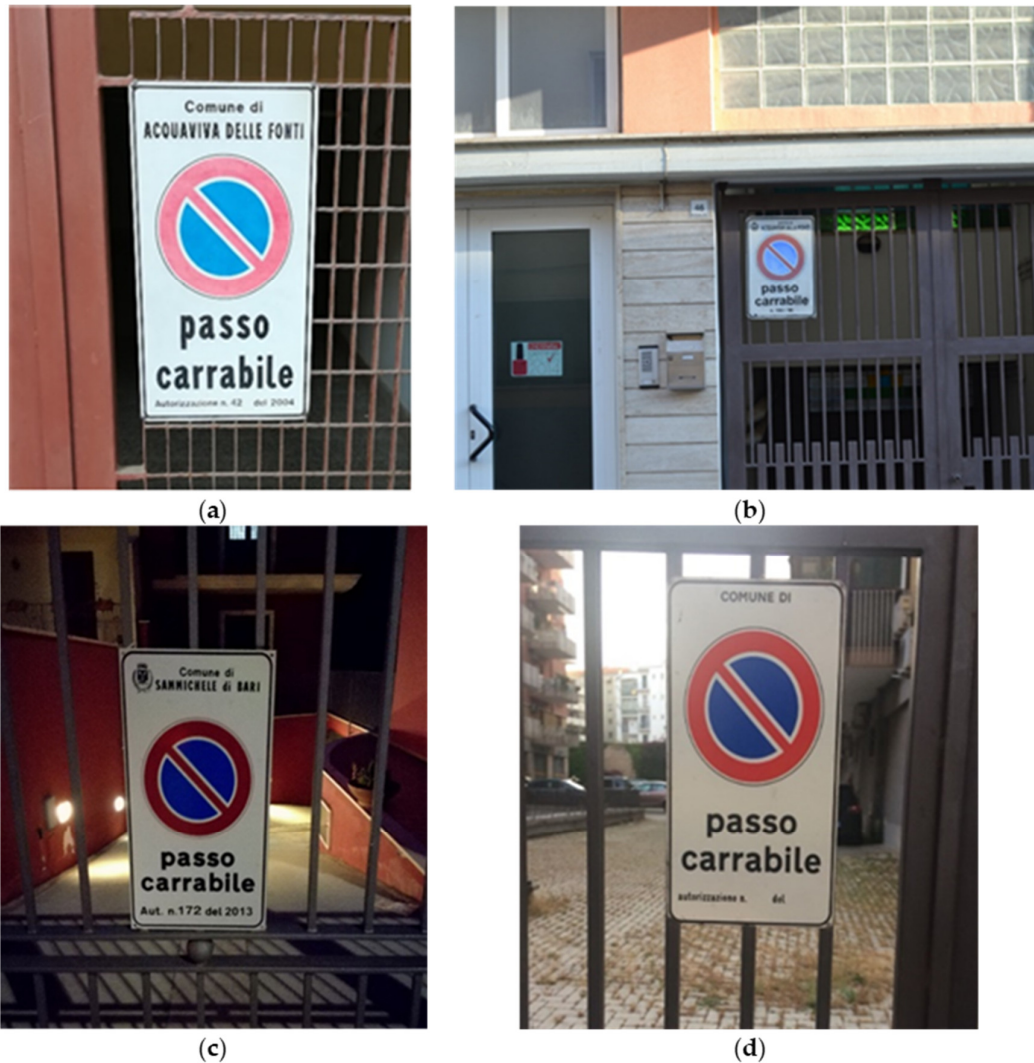
Figure 3. Examples from the classes of the tow-away road sign image dataset: (a) C1: Close distance and simple scenario; (b) far distance, complex scenario; (c) poor lighting; (d) false road sign or license code featuring missing/wrong information.
