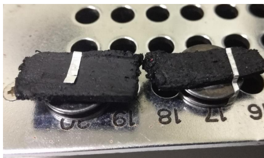
Figure 15. Conductive polymer samples prepared for microscopic analysis.
