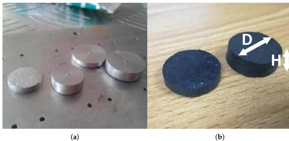
Figure 12. Fabrication of the sensor pills: (a) spacers to alter the thickness values of the pills; (b) conductive polymer pills after the fabrication.
