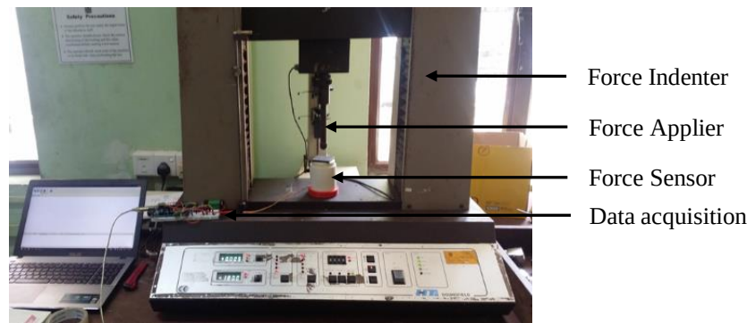
Figure 20. Force indenter is used for sensor characterisation.
