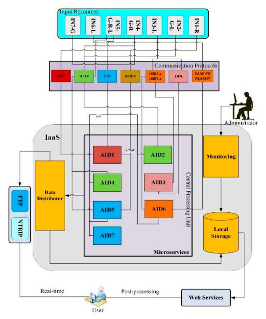
**Figure 2.** Block diagram of the designed information and communication technology (ICT) technical architecture.
