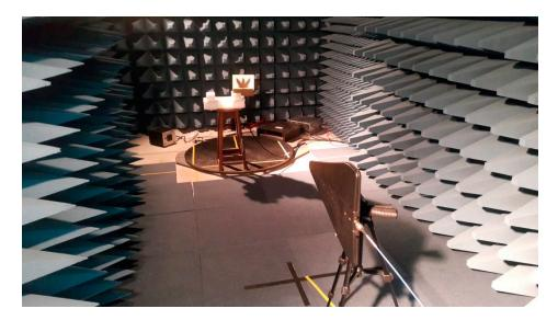
Figure 12. Photograph of the gain measurement test experimental setup.
