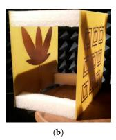
**Figure 27.** Manufactured bio-inspired PMA: (a) without metamaterial superstrate [26]; (b) with metamaterial superstrate.
