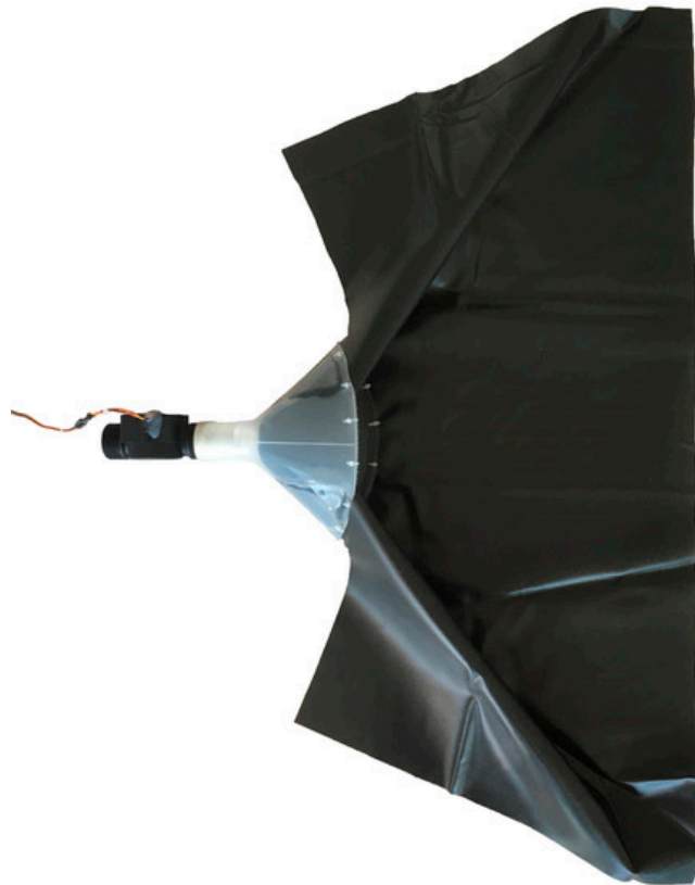
Figure 8. Top view of the flow sensor with funnel and tarp (2017 field season setup).
