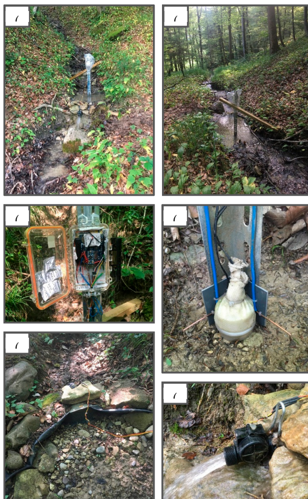
Figure 11. Field setup of the multi-sensor monitoring system (2017 field season): (a) upstream view of the monitoring system in a flowing stream, (b) downstream view of the monitoring system in a flowing stream, (c) the waterproof box, containing the microcontroller board and data logger shield
