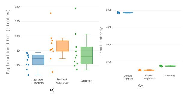
**Figure 13.** A comparison of the exploration with different heuristics: Nearest neighbour, octomap sector order, and closest surface frontier. Each heuristic was run 10 times. (**a**) Distribution of the time the system needs to complete the exploration task and (**b**) total entropy at the end of each run.
