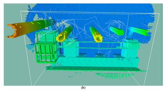
**Figure 17.** A comparison of the final map with different heuristics. The path is represented as a white line. The search space is represented as a white box. The measurements are incorporated into the world representation even if they are outside the navigational bounds defined by the operator. (**a**) Nearest neighbour and (**b**) surface frontier.
