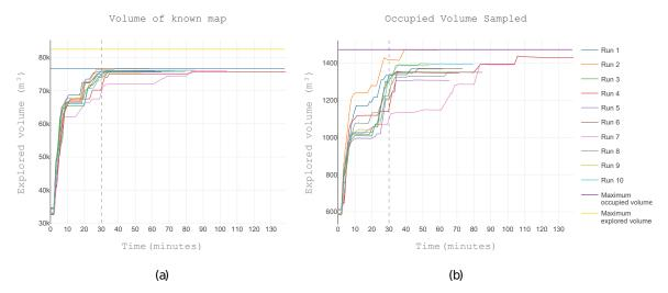
**Figure 14.** The volume explored in 10 runs. (**a**) Rate of exploration: Free and occupied are combined. (**b**) Coverage of the occupied volume.
