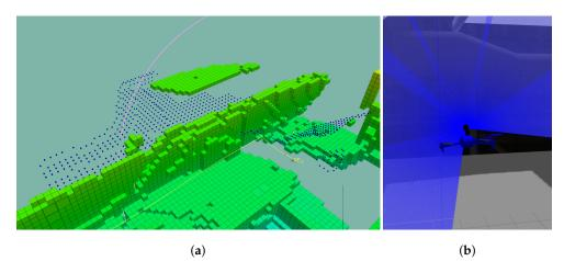
**Figure 3.** Neighbour generation, according to the sensor range. (**a**) The frontiers in blue could not be sampled as the only known space is above and the laser scanner has a blind spot below due to the 270° scan angle. (**b**) The blue rays illustrate the range of the sensor. The scan angle is pointed upwards.
