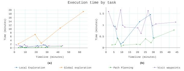
**Figure 11.** The execution time the mission manager spent in each task, in one run with a circular iterator. (a) All four tasked scaled together and (b) just local exploration, path planning, and visit waypoints.
