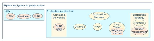
**Figure 6.** The architecture applied to the case of an AUV (Autonomous Underwater Vehicle). The changes are highlighted in orange and are primarily at the hardware level.
