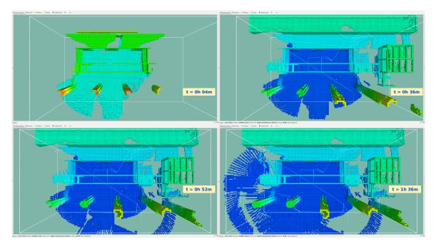
**Figure 16.** The evolution of occupied space present, throughout a mission cycle. A snapshot is taken at the end of the initial manoeuvre and every 30 min after that. The last snapshot shows the final map. The light blue line illustrates the path taken by the vehicle. The white outline represents the search space defined by the operator.
