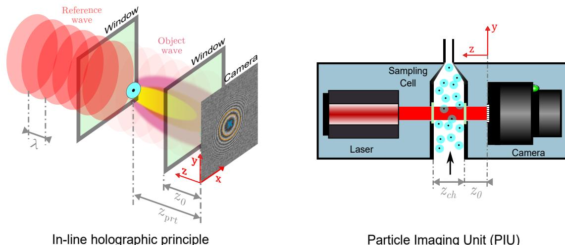
**Figure 1.** Left: in-line holographic principle where a single particle creates a fringe pattern at the camera plane. The detection is based on recognizing the set of concentric rings (in orange & blue); Right: schematic of the in-line holographic counting unit, subsequently called Particle Imaging Unit (PIU).
