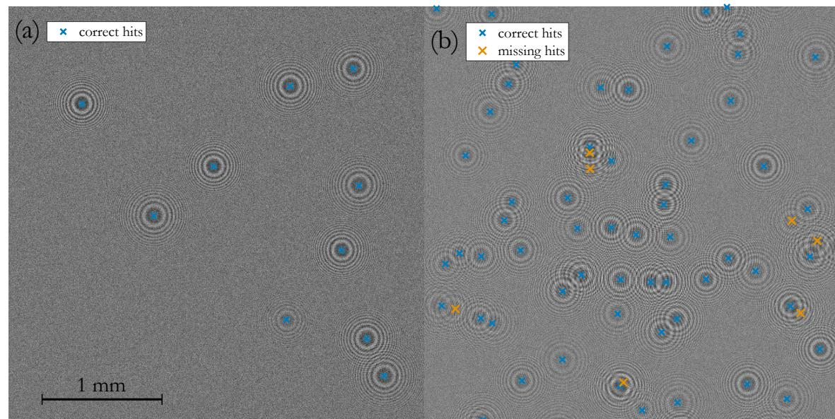
**Figure 4.** Zoomed segments of frames at: (a) low particle density of  $78 \frac{\#}{frame}$  and no missing hits; (b) medium particle density of  $273 \frac{\#}{frame}$  with missing hits. Because of intrinsic higher speckle noise in the right frame segment, the contrast is lower while the background noise level is increased.
