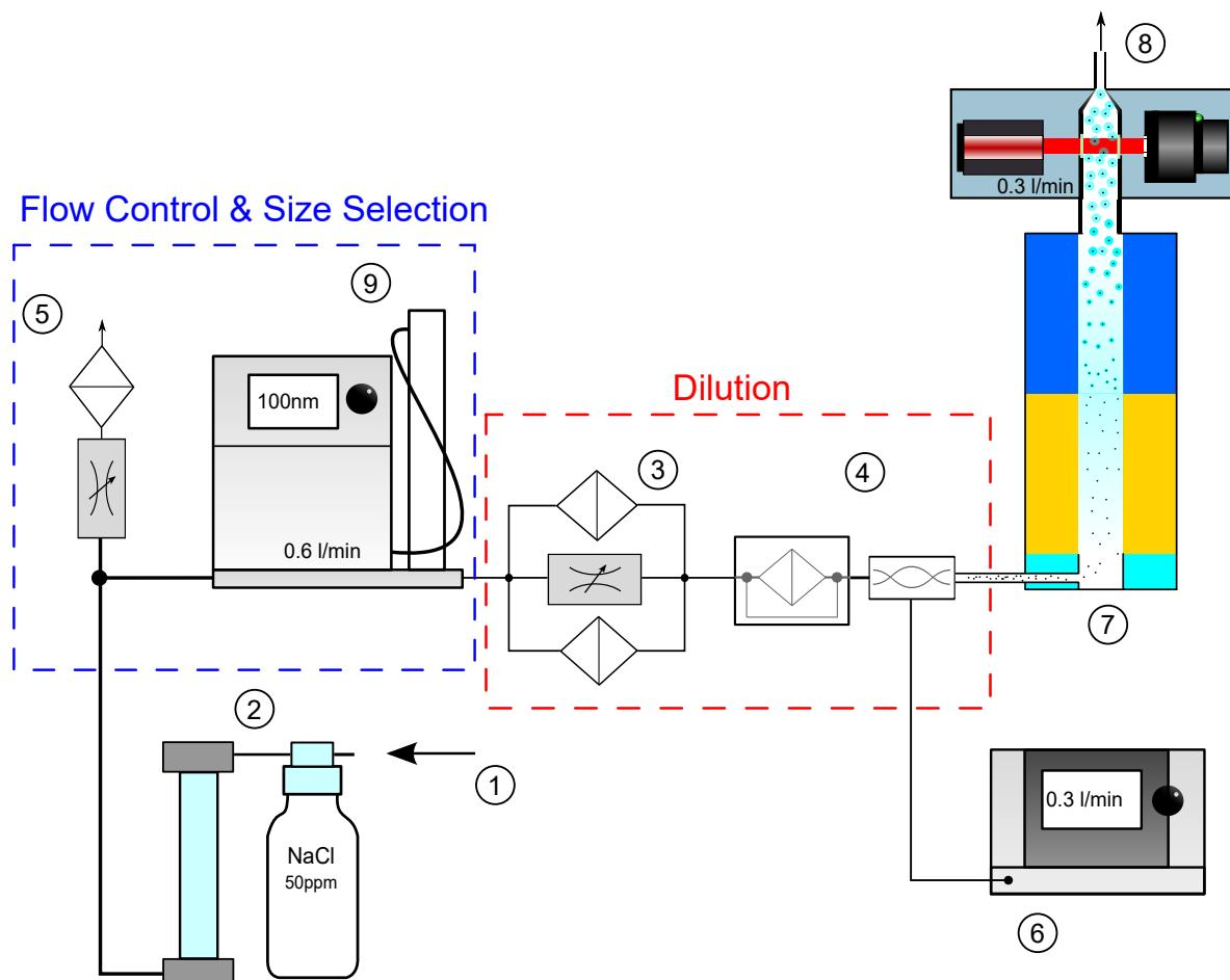
**Figure 5.** Experimental Setup for measurement of particle concentration.
