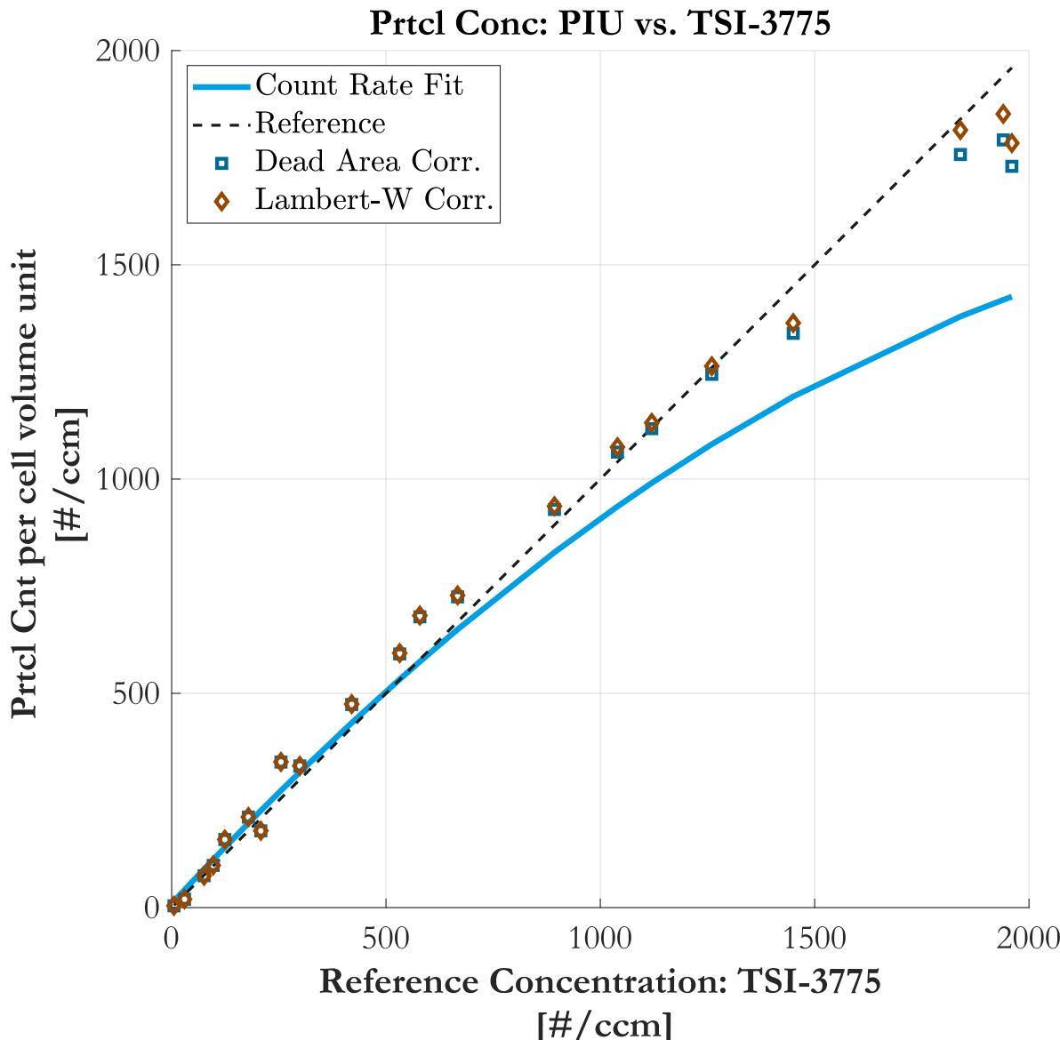
**Figure 8.** Comparison of particle number concentration obtained by the Particle Imaging Unit (PIU) and the TSI-3775 (uncorrected in blue). The concentration is coincidence-corrected by *Dead Area* and *Lambert-W* correction, both with a mean dead area diameter of  $\delta_d = 60$  pxl.
