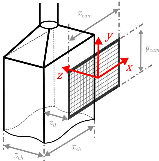
**Figure 2.** Sampling channel geometry of the PIU.
