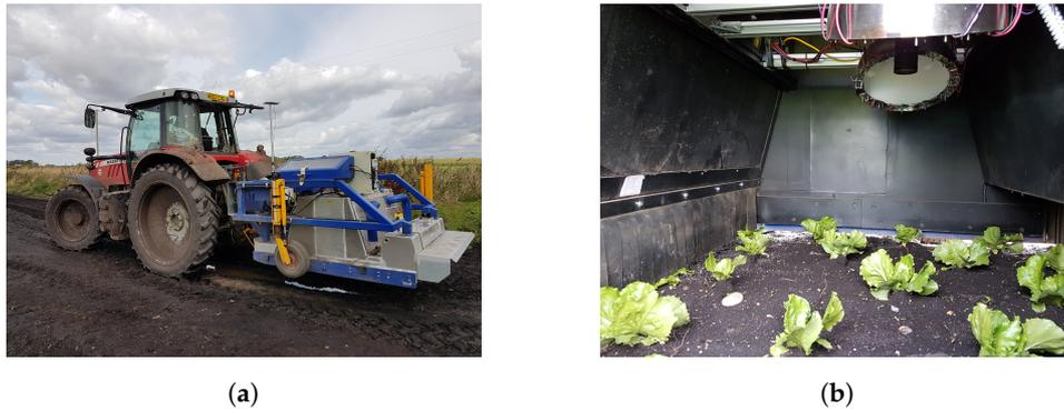
**Figure 1.** The system in field trials. (a) The system mounted to the rear of the tractor. (b) The sensor system in-field.
