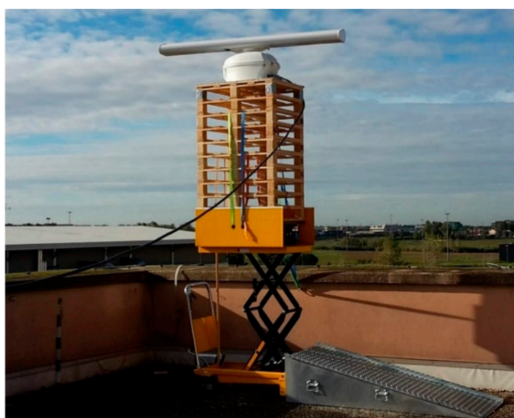
Figure 1. The Simrad/Navico SRT Radar and its lifter on the top of the Information Engineering building (Tor Vergata University).
