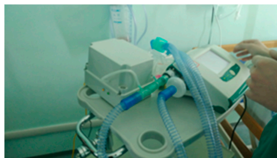
Figure 10. Breath Analyzer Module connected to bi-tube breathing circuit in real operating condition during clinical experimentation in hospital setting.
