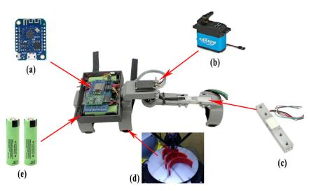
**Figure 3.** Components of the exoskeleton of a one degree of freedom (DOF) EXOMedical: (**a**) ESP8266 Wireless microcontroller; (**b**) 15 kg servo motor; (**c**) Load cell up to 25 kg; (**d**) 3D printed parts in PLA; (**e**) Two 18,650 lithium batteries of 3.7v 3400 mah each.
