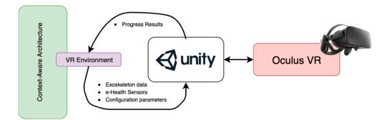
**Figure 5.** Main components of the virtual reality environment based on the Unity 3D engine and the Oculus system.
