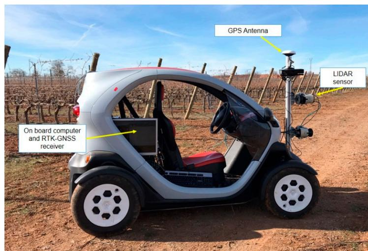
**Figure 1.** Electric mobile platform comprising light detection and ranging (LiDAR) laser scanner and GPS-RTK receiver mounted on a lightweight extruded aluminum with adjustable height. Data is captured on an on-board computer.
