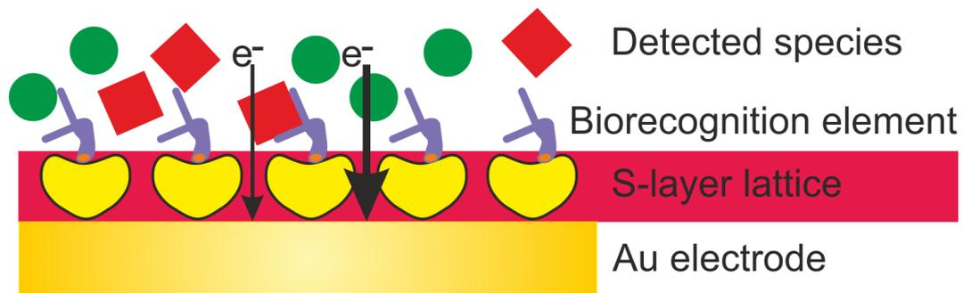
**Figure 2.** Schematic drawing (not drawn to scale) of an electrochemical biosensor with an S-layer lattice as intermediate layer for linking biorecognition elements to the Au (gold) electrode surfaces.
