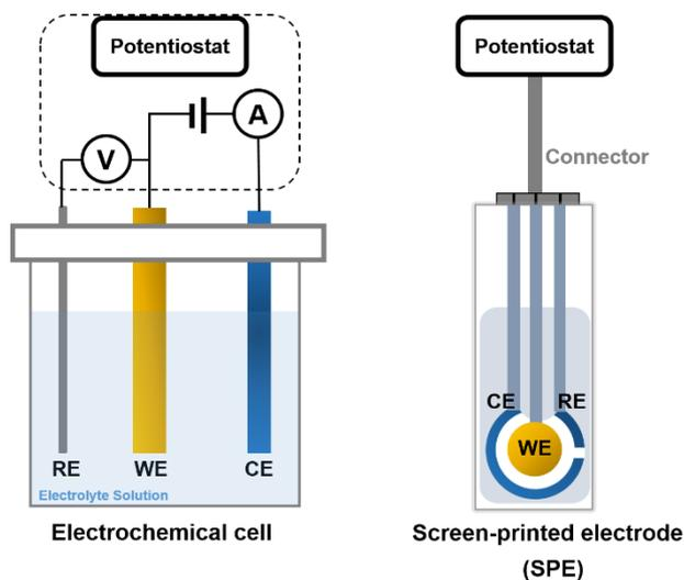
**Figure 5.** The two types of electrochemical biosensors with three electrodes: reference (RE), working (WE), and counter (CE) connected to a potentiostat.
