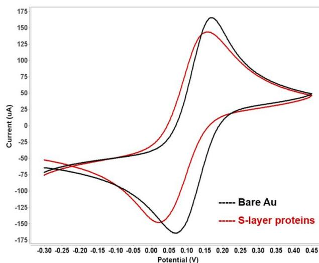
**Figure 4.** Cyclic voltammogram of the bare and the S-layer protein-coated gold electrode in 10 mM  $[\text{Fe}(\text{CN})_6]^{3-/4-}$  containing 100 mM KCl at a scan rate of 50 mV/s.
