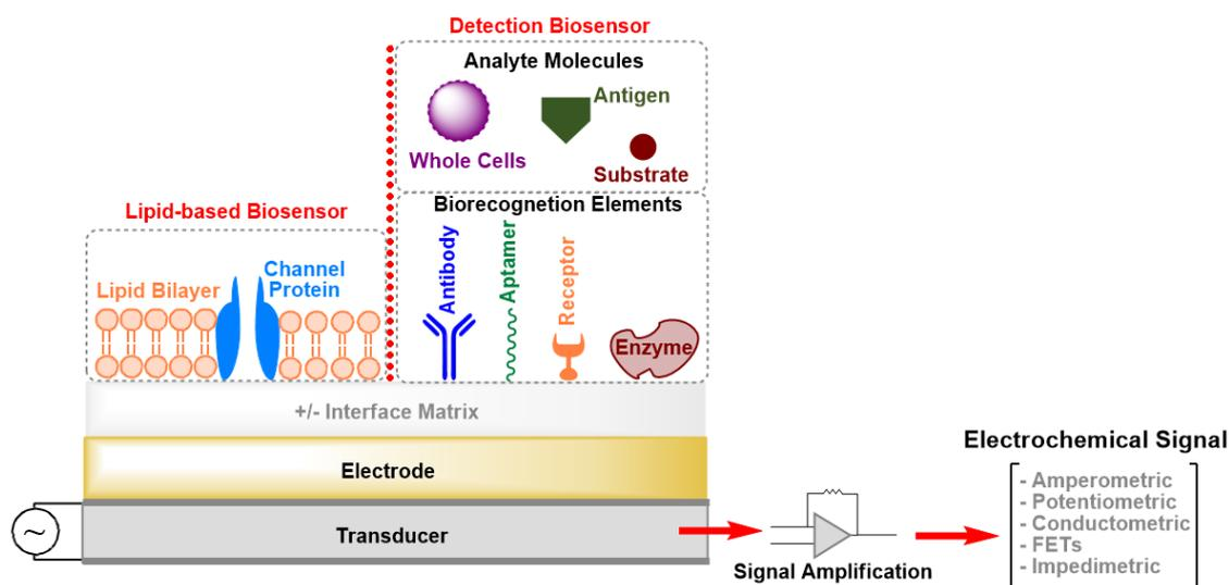
**Figure 1.** Schematic drawing (not drawn to scale) of the elements of an electrochemical biosensor. FETs: Field-Effect Transistors.
