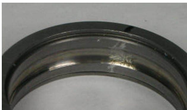
Figure 7. Outer race fault.
