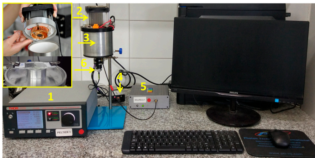
Figure 1. A stationary cure monitoring system was composed of a microcomputer-controlled miniature spectrometer (EPP2000C from StellarNet, Inc., Tampa, FL, USA): 1—thermostat (Thorlabs, Inc., Newton, NJ, USA), 2—Peltier cell with heatsink, 3—measuring chamber, 4—power supply, 5—spectrometer (StellarNet, Inc., Tampa, FL, USA), 6—UV-LED diode.
