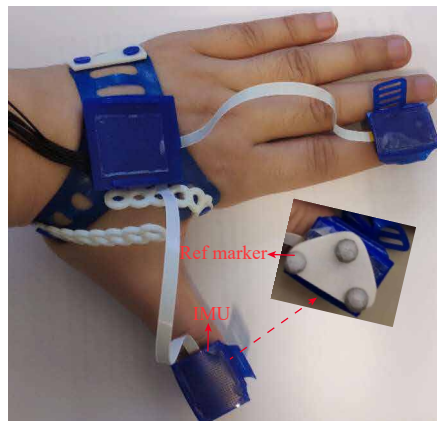
Figure 1. IMUs on the dorsal side of the hand and fingertips. The inset shows the cluster of optical markers used on top of each IMU for reference measurement of segment orientations using the optical VICON system. Every cluster contains three markers, which determine a 3D coordinate frame.
