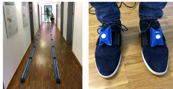
Figure 3. Gait data recording set-up. Left: the 10 m OptoGait walkway. Right: the IMUs were fixed on top of the shoes.
