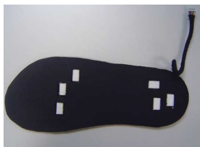
Figure 8. Insole with six textile sensors [6].
