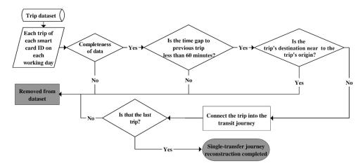
Figure 1. Process to construct single-transfer travel journeys.
