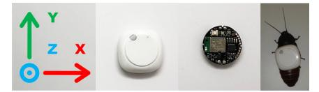
**Figure 7.** MetaMotion C Sensor Board: From left to right: (1) Coordinate frame of MetaMotion C sensor board (this is the body frame of our algorithm); (2) 3D-printed MetaMotion C case; (3) MetaMotion C PCB; (4) The IMU (inside the case) is mounted to the thorax of the biobot with the +Y direction of the IMU facing in the direction of the biobot's antennae.
