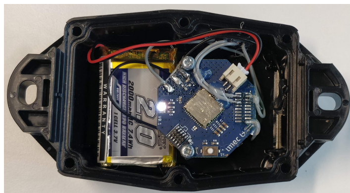
Figure 5. Our multi-RAT LPWAN device is able to switch between Sigfox, LoRaWAN, and DASH7 communication.
