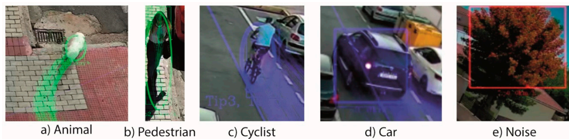
Figure 11. Classification of the elements: (a) animal, (b) pedestrian, (c) cyclist, (d) car, (e) noise.
