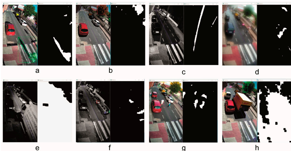
Figure 7. Background subtraction method: (a) sunny weather, (b) windy weather, (c) rainy weather, (d) light rainy fog, (e) very abrupt lighting change, (f) slight lighting change, (g) blur capture, (h) camera vibrations.
