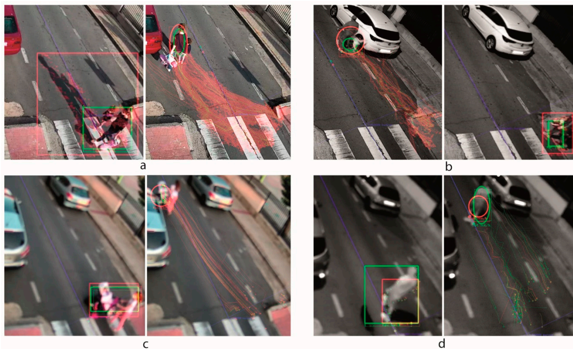
Figure 10. Tracking of points defined by FAST (red) and GFTT (green) detectors: (a) with good visibility during the day, (b) with good visibility at night, (c) adverse visibility conditions during the day, (d) adverse visibility conditions at night.
