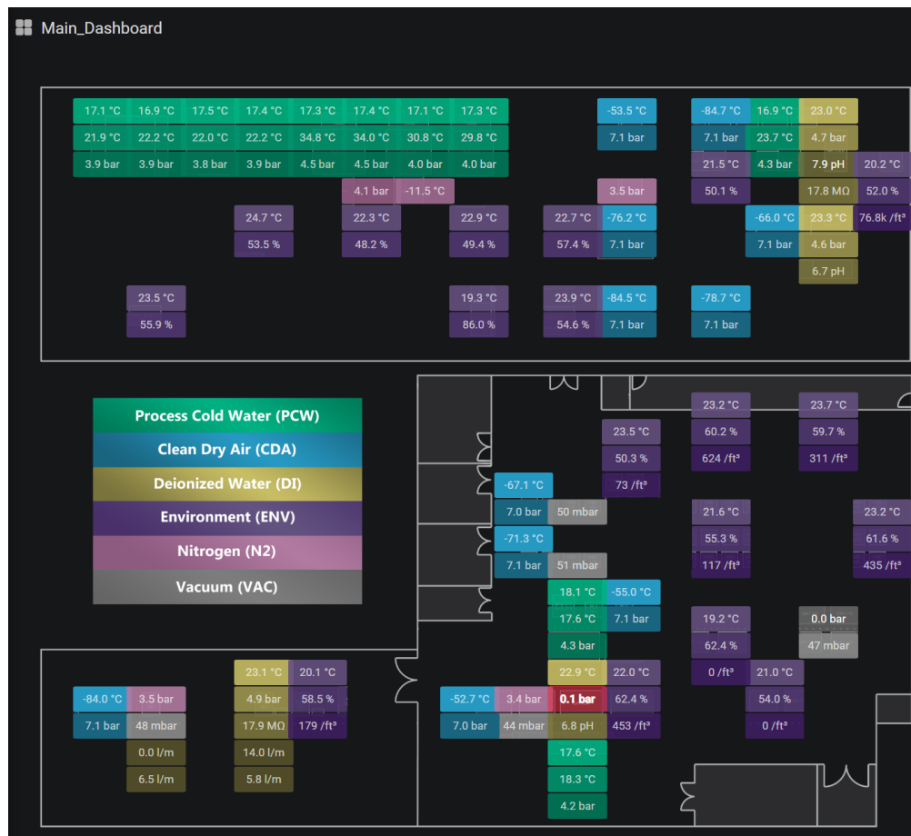
Figure 6. Using the visualization tool to map and analyze the state of the sensors in the industrial plant.
