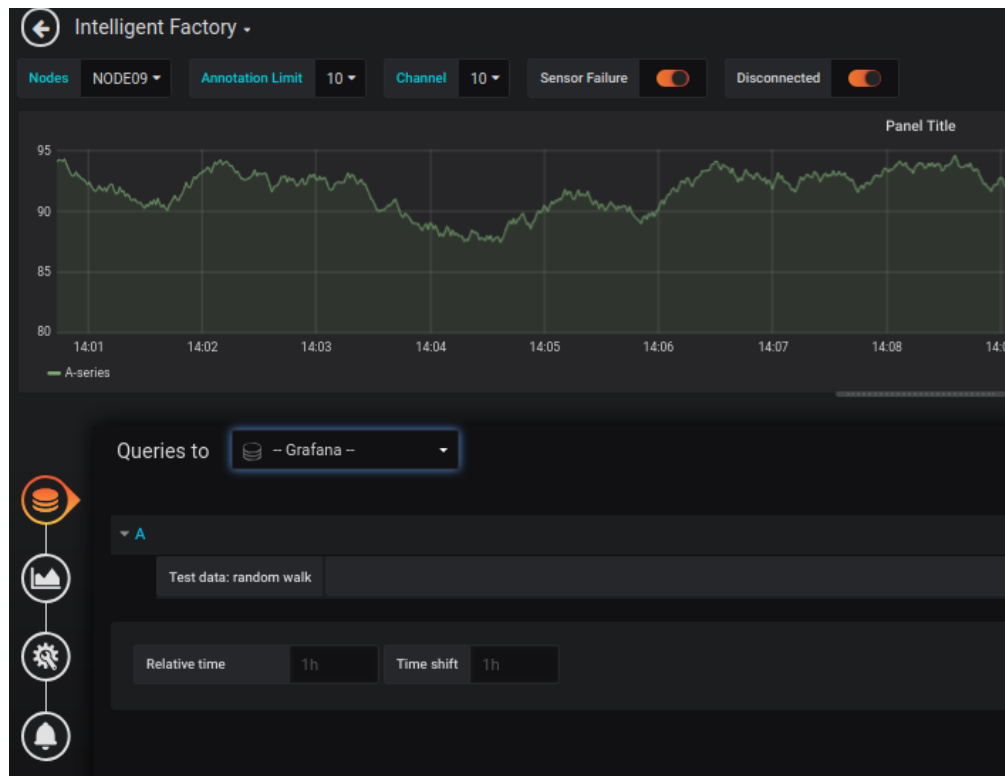
Figure 7. Example of observing historical data of a particular sensor. The graphical interface allows system administrators to configure different threshold-based warning levels, enabling push notifications that trigger actions to the support team.
