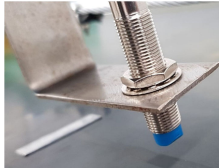
Figure 6. Inductive sensor at the measuring point.
