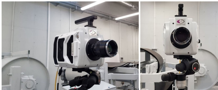
Figure 9. View of the Phantom v2640 camera at the measurement location.
