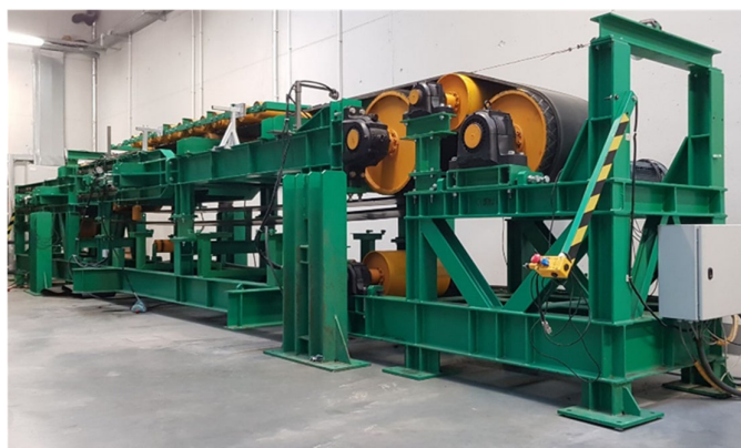
Figure 1. Intermediate belt drive test rig.
