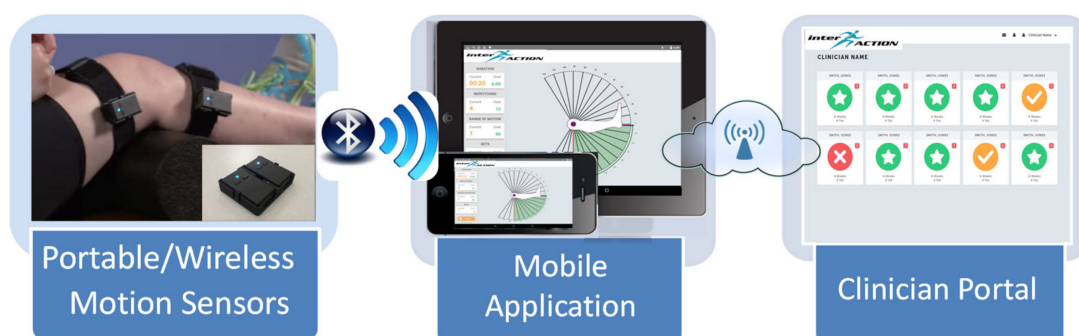
Figure 1. Conceptual flowchart of the interACTION platform: (1) inertial measurement units (IMUs) attached to the patient’s thigh and shank using neoprene straps and 3D-printed cases, (2) mobile application utilized by the patient to complete their prescribed home exercises, (3) screenshot of clinician portal depicting the patient dashboard which is utilized by the physical therapist to manage the patient’s rehabilitation remotely.
