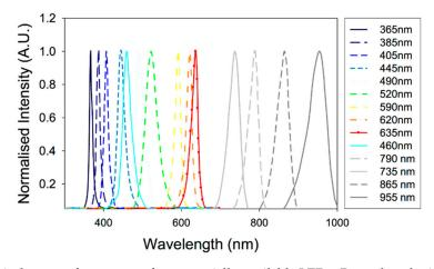
**Figure 4.** Optical spectra for a range of commercially available LEDs. Reproduced with permission from T. J. Allen and P. C. Beard, Biomedical Optics Express, Vol.7, Article ID1260, 2016; licensed under a Creative Commons Attribution (CC BY) license.
