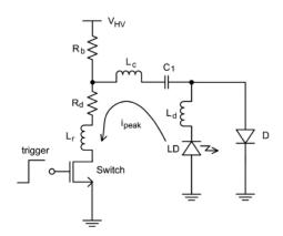
**Figure 11.** Typical laser driver circuit. Reproduced with permission from H. Zhong, T. Duan, H. Lan, M. Zhou, F. Gao, Sensors, Vol.18, Article ID2264, 2018; licensed under a Creative Commons Attribution (CC BY) license.
