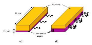
**Figure 13.** Schematic diagram of (**a**) a standard diode bar and (**b**) a multiple active region diode bar. Adapted with permission from Proc. SPIE 9887, Biophotonics: Photonic Solutions for Better Health Care V, 98872B (2016). Copyright 2016 Society of Photo-Optical Instrumentation Engineers (SPIE).
