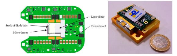
**Figure 12.** Schematic diagram of the diode laser source showing implementation of the laser diode within the driver board (**left**). An ultra-short pulse laser source integrating a mini-laser diode providing 1.7 mJ in pulses as short as 40 ns from Quantel, France (**right**). Adapted with permission from Proc. SPIE 9887, Biophotonics: Photonic Solutions for Better Health Care V, 98872B (2016). Copyright 2016 Society of Photo-Optical Instrumentation Engineers (SPIE).
