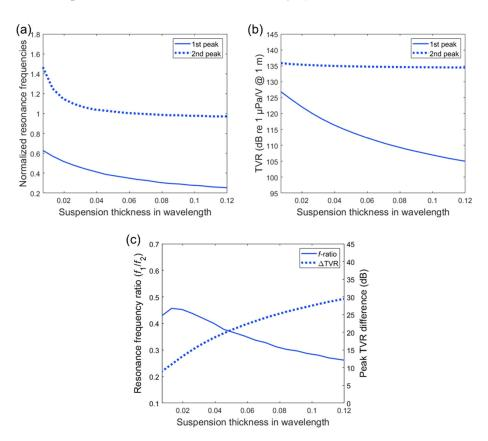
**Figure 5.** Transmitting characteristics as a function of suspension thickness. The thickness dimension is presented in wavelength and the frequency values are normalized by the fundamental longitudinal resonance frequency  $f_2$ : (a) normalized resonance frequency variation; (b) TVR peak variation; (c) the variation in resonance frequency ratio ( $f_1/f_2$ ) and TVR difference.
