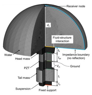
Figure 2. A finite element model (2-D axis-symmetric model) of the rear-mounted Tonpilz transducer.
