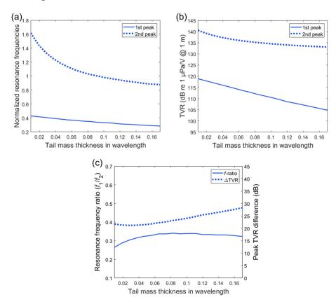
**Figure 6.** Transmitting characteristics as a function of the tail mass thickness. The thickness dimension is presented in wavelength and the frequency values are normalized by the fundamental longitudinal resonance frequency: (a) normalized resonance frequency variation; (b) TVR peak variation; (c) variation in resonance frequency ratio  $(f_1/f_2)$  and TVR difference.
