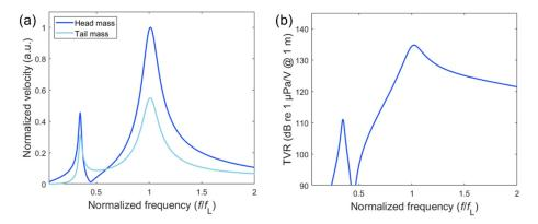
**Figure 9.** The comparison between the (a) velocity spectra (head mass and tail mass) and (b) TVR spectrum calculated by the distributed circuit model (basic design).
