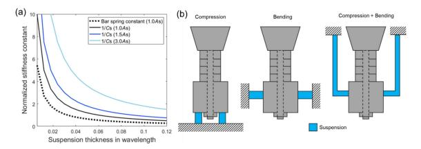
**Figure 8.** Material and design of a suspension: (a) effective stiffness as a function of suspension thickness. The larger cross-sectional areas  $(1.5A_s \text{ and } 3.0A_s)$  yield higher stiffness; (b) suspension design examples (4-layer stacked piezo-element as an example). The same effective stiffness can be designed by adjusting the suspension structure and material.
