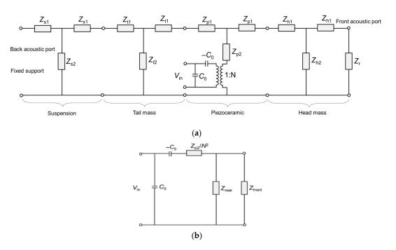
**Figure 3.** Schematic representation of the equivalent circuit of the rear-mounted Tonpilz transducer. The load elements are defined in Table 2: (a) distributed equivalent circuit model; (b) rearrangement of the circuit in (a) with combined loads. All load impedance elements are referred to as the electrical side.
