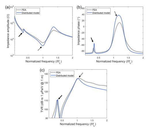
**Figure 4.** Equivalent circuit and finite element analysis (FEA) simulation of the electrical impedance and the transmitting voltage response (TVR) of the rear-mounted design: (a) impedance amplitude spectra; (b) impedance phase spectra; (c) TVR spectra. The suspension-induced peaks are marked by solid arrows while the fundamental resonance peaks are depicted by dotted arrows.
