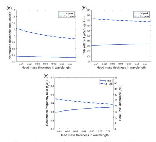
**Figure 7.** Transmitting characteristics as a function of the head mass thickness. The thickness dimension is presented in wavelength and the frequency values are normalized by the fundamental longitudinal resonance frequency: (a) normalized resonance frequency variation; (b) TVR peak variation; (c) variation in resonance frequency ratio  $(f_1/f_2)$  and TVR difference.
