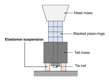
**Figure 1.** Schematic representation of a rear-mounted Tonpilz projector (4-layer stacked piezo-element as an example). A tail mass is supported by an elastomer suspension to generate a low-frequency resonance below the fundamental longitudinal mode resonance.
