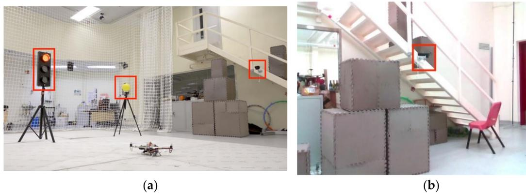
**Figure 9.** Images of the experiments conducted in the indoor environment. (a) Three objects, including a traffic light, a bulb, and a CCTV for inspection mission are marked with red rectangles. (b) The target device CCTV is shown outside of the range of the motion capture system.
