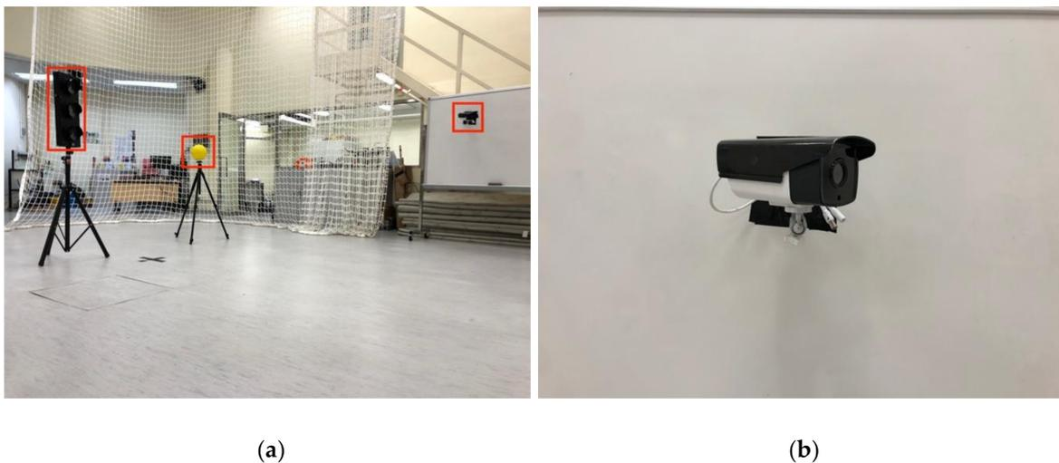
**Figure 12.** Picture of the visual-inertial odometry flight experiment. (a) Three objects: traffic light, bulb, and CCTV for inspection mission are marked with red rectangles. (b) The target device CCTV is fixed on a whiteboard with tapes.
