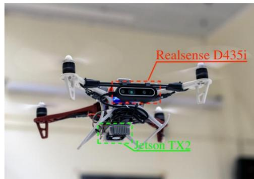
**Figure 1.** The unmanned aerial vehicle (UAV) inspection system during flight.
