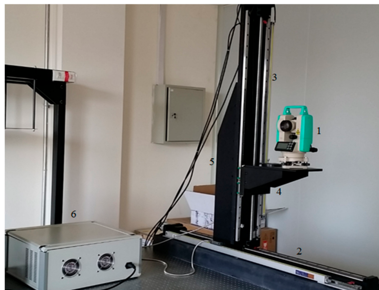
Figure 8. The ultra-high precision camera calibration platform.
