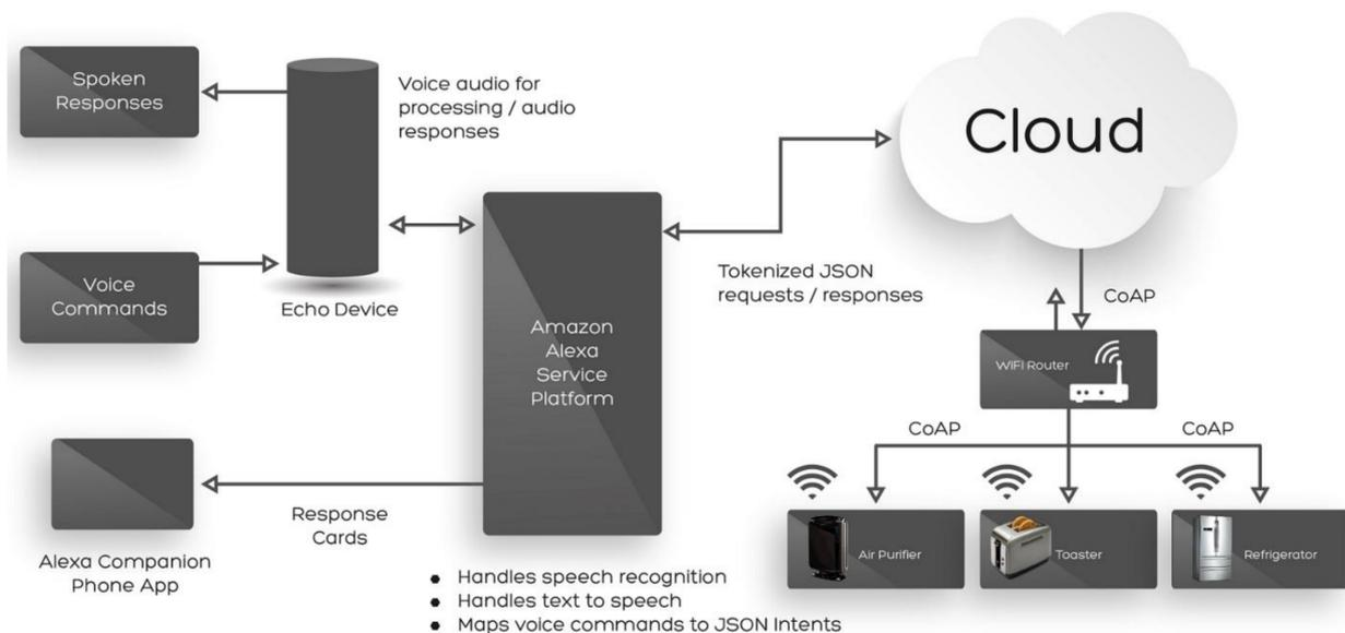
**Figure 1.** Architecture of a voice assistant (Alexa) (<https://www.faststreamtech.com/blog/amazon-alexa-integrated-with-iot-ecosystem-service/>). (access on 10 February 2021) [8].
