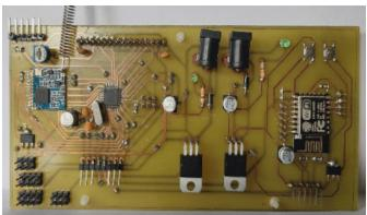
Figure 3. LoRa-based gateway.
