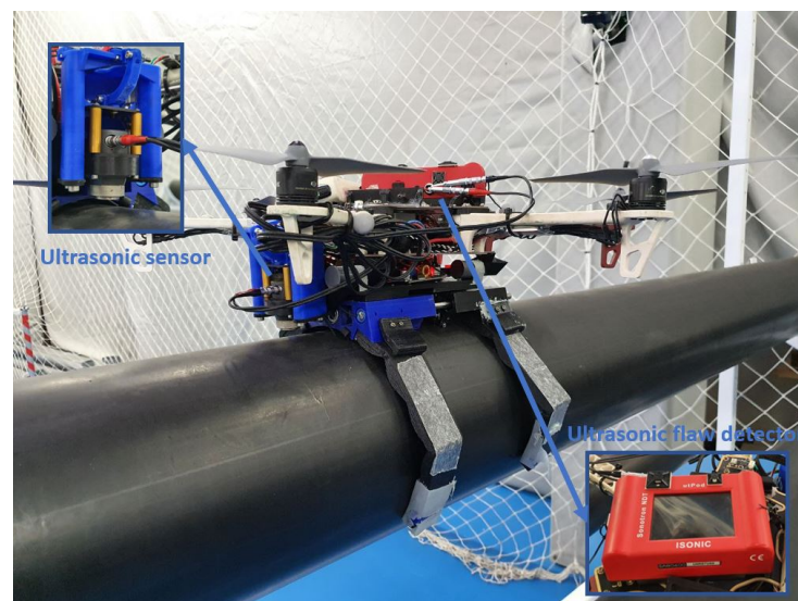
Figure 18. The image shows the complete system with an ultrasonic sensor and the flaw detection computer.
