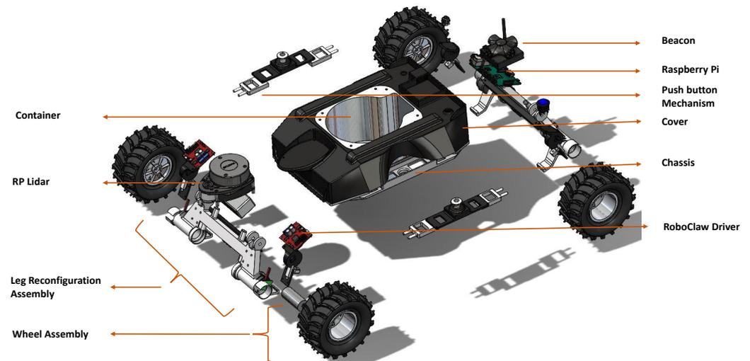
**Figure 1.** Mechanical components.
