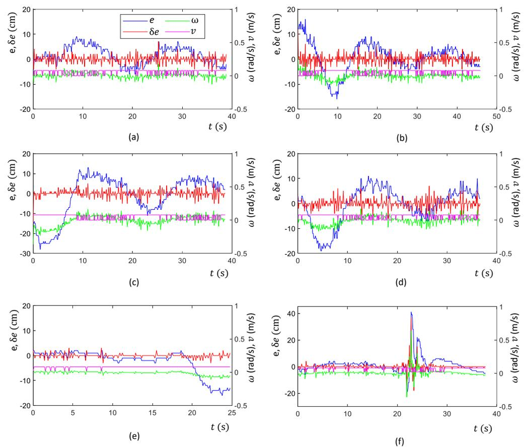
**Figure 13.** Variation of inputs and outputs of decision-making process of navigating in the middle of a drain in the considered test scenarios. (a) Scenario ‘a’, (b) Scenario ‘b’, (c) Scenario ‘c’, (d) Scenario ‘d’, (e) Scenario ‘e’, and (f) Scenario ‘f’.
