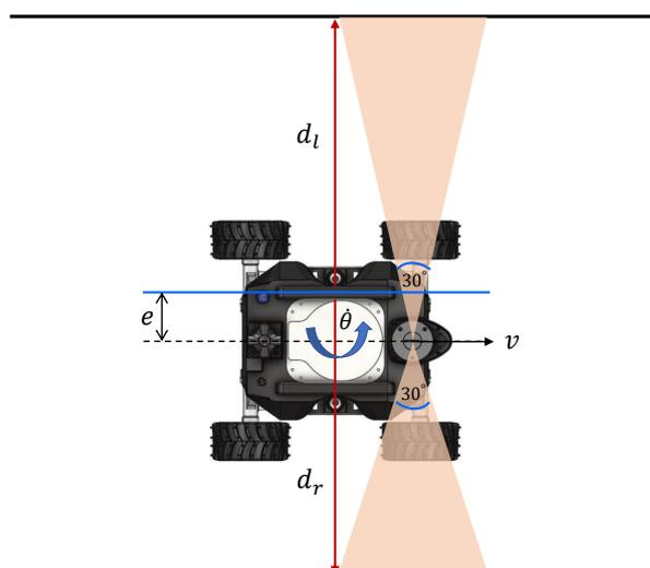
Figure 9. Principle of navigating in the middle of a drain.
