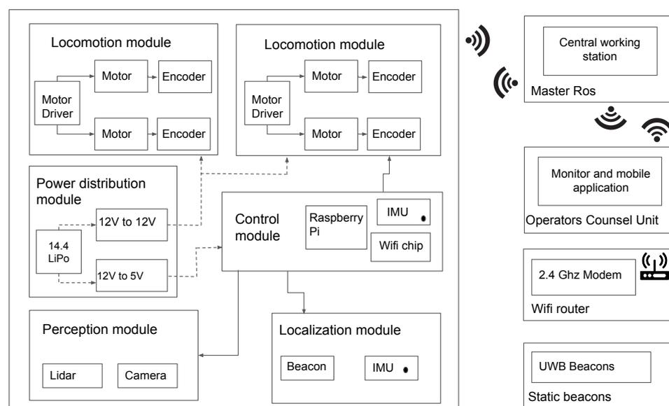
Figure 6. Control Architecture.
