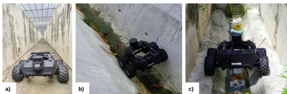
**Figure 3.** Adaptability of the robot to various drain scenarios. (a) In a drain with a flat floor (b) In a drain with a curved bottom (c) In a cut-off drain
