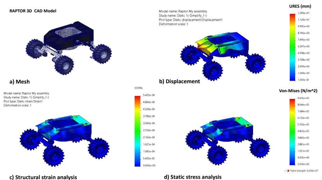
**Figure 5.** Static structural analysis (a) Tetrahedral mesh of Raptor 3D model (b) Static Displacement analysis (c) Strain Analysis results (d) Von Mises stress in  $N/m^2$ .
