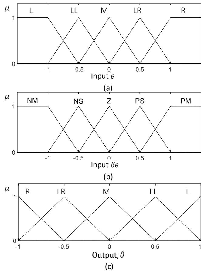
**Figure 10.** Input and output membership functions of fuzzy inference system. (a,b) The input membership functions. (c) The output membership function. The fuzzy labels are defined as R: Right, LR: Little Right, M: Middle, LL: Little Left, L: Left, NM: Negative Medium, NS: Negative Small, Z: Zero, PS: Positive Small, and PM: Positive Medium. It should be noted that the membership functions are given in normalized scales.
