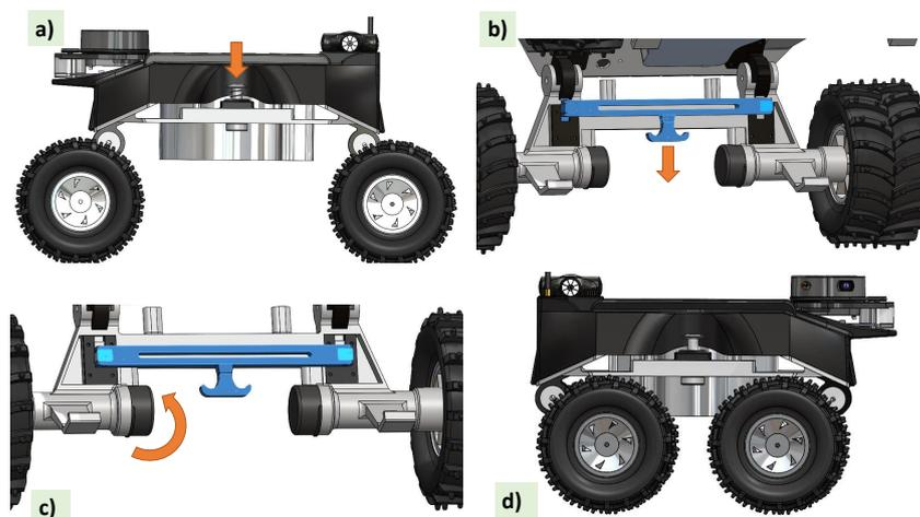
**Figure 2.** Steps of the reconfiguration. (a) Push button pressing to open the provision to insert and hold the pin (b) Pulling the lock open when triggering the pull lever (c) Adjusting the wheel assemblies (d) New wheel assembly configuration
